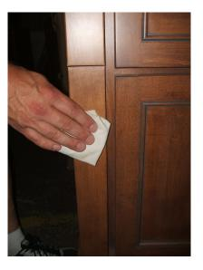
5. Inspect entire part for any defect, such as rub marks.
