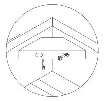
**6.** Put the screw in the hole of the toe board that was not removed, (this will help hold it in place as you put the screw in the new toe board.
