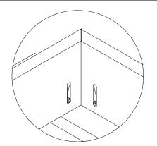
**5.** Hold the toe board in place and replace the screws that were removed earlier.
