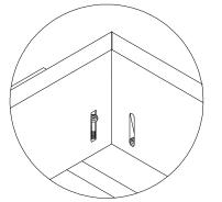
**3.** Remove the screws from the damaged toe board and remove it.
