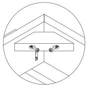
**2.** Remove the screws from the corner blocks with a Philips screwdriver.
