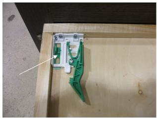
To adjust the drawer front, for level move this lever either to the front or to the back.
