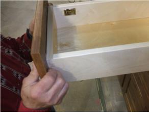
Pull the drawer front out to the end of the glide. Push drawer to the right to adjust to left side. Push the drawer to the left to adjust to right side. Some times it takes the closing the drawer firmly two or three times to adjust the glides at the back.
